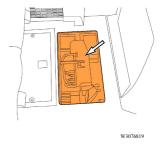
If the fuse fails, it should be replaced by an 50A fuse. Never insert a fuse of a higher amperage rate.
