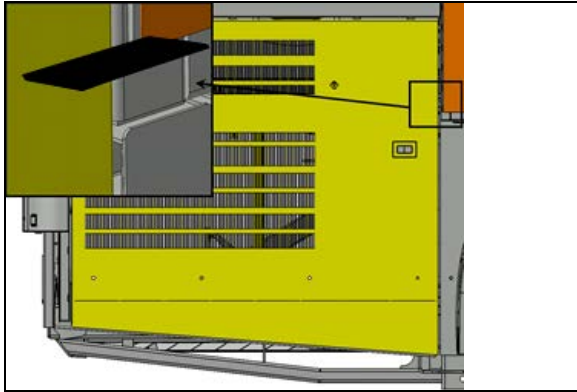
FIGURE 118: USE A RULER (SHOWN IN BLACK) TO CHECK THAT SURFACES ARE EVEN
