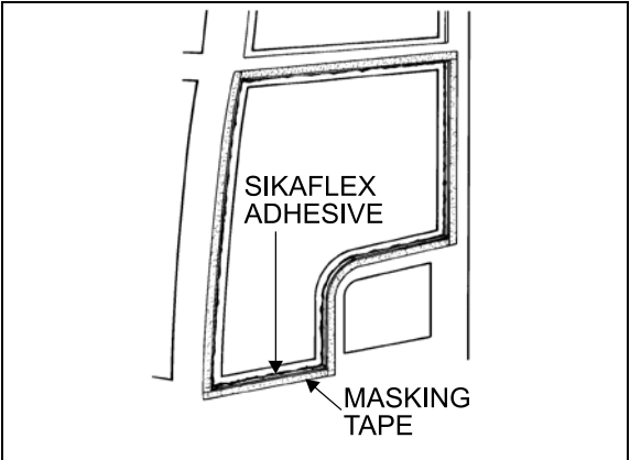
FIGURE 46: ADHESIVE-MOUNTED WINDOW 18081
