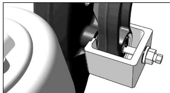
FIGURE 15: INSTALLING EXTRACTOR TOOL
