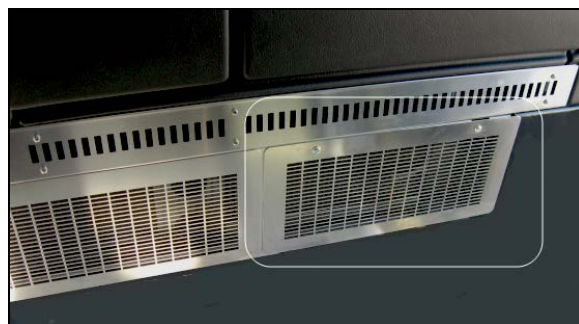
ACCESS TO DRIVER'S HVAC UNIT AIR FILTER
