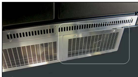
ACCESS TO DRIVER'S HVAC UNIT AIR FILTER
