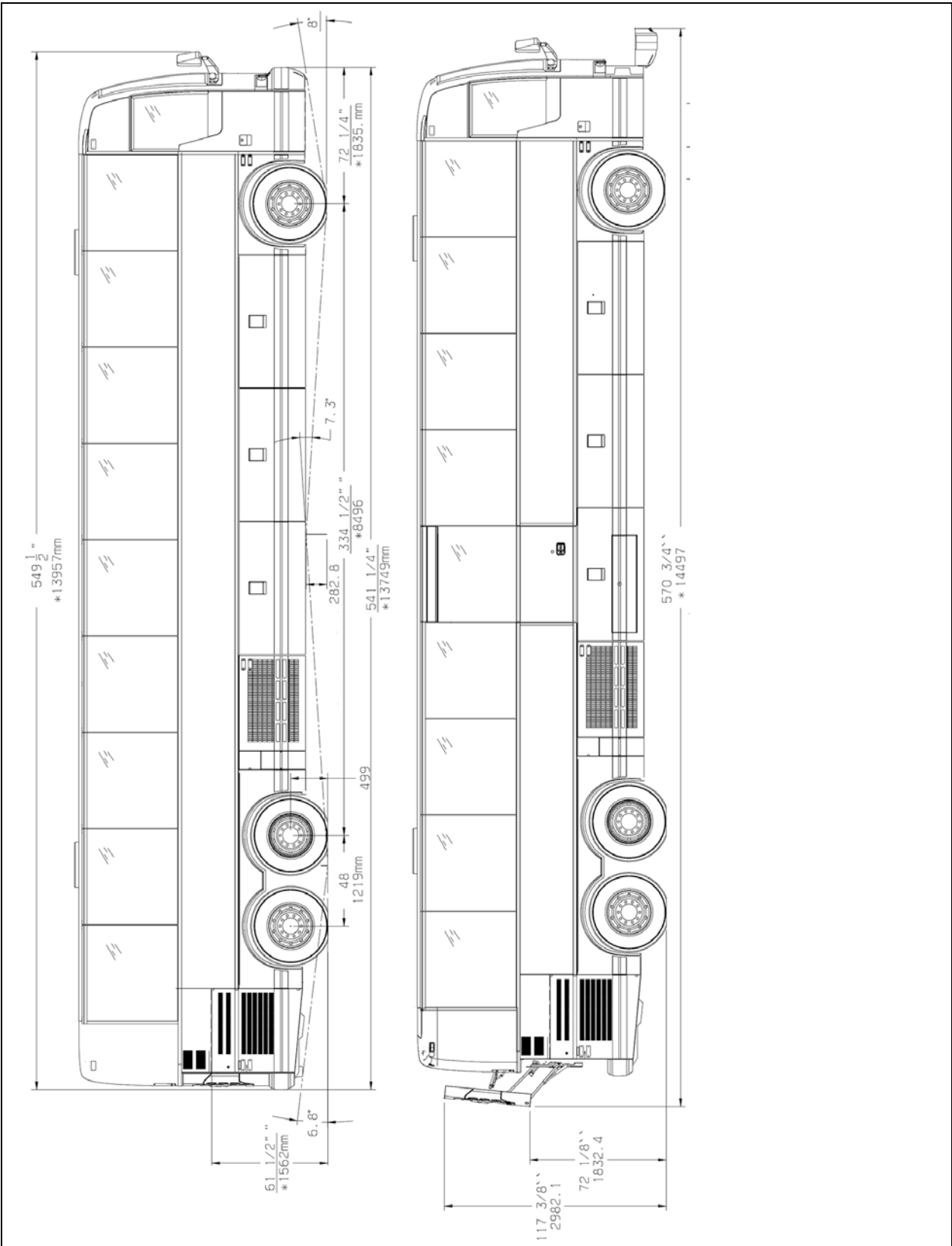
X3-45 OVERALL DIMENSIONS (SIDE ELEVATION)
