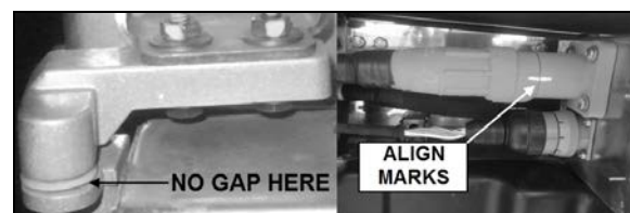
FIGURE 26: INSTALLED HINGE & MAIN CONNECTOR
