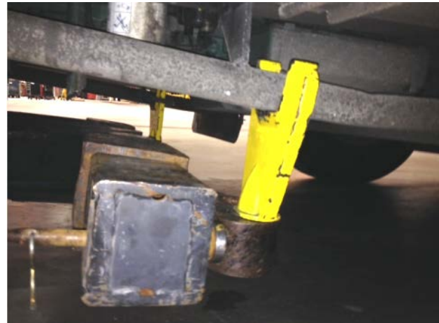
FIGURE 61 : PROPER LOCATION WHEN LIFTING THE SIDE MEMBERS
