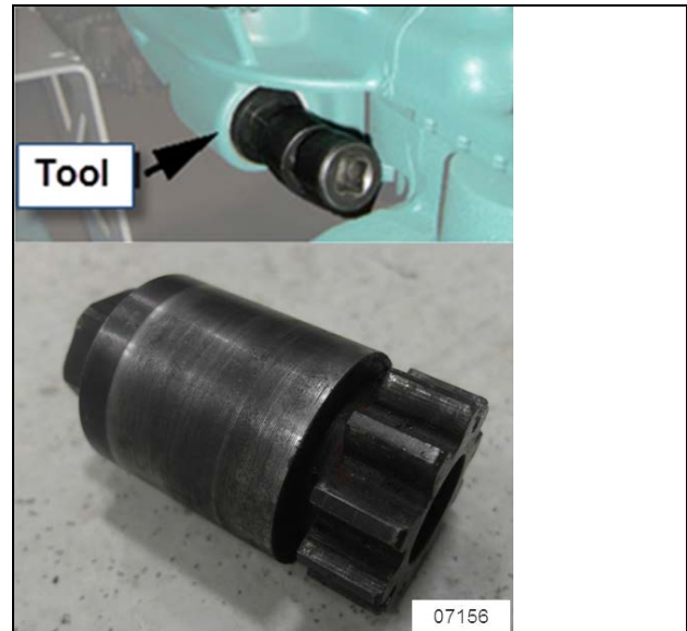
FIGURE 10: VOLVO ENGINE TURNING TOOL #88800014
