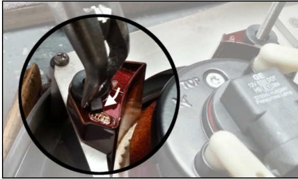
FIGURE 73: UNLOCK THREADED ROD
