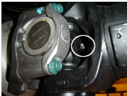
FIGURE 5: BEARING LUBRICATION ZIRK
