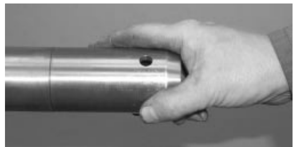
FIGURE 9: INSERTION TOOL PREVOST P/N 491115
