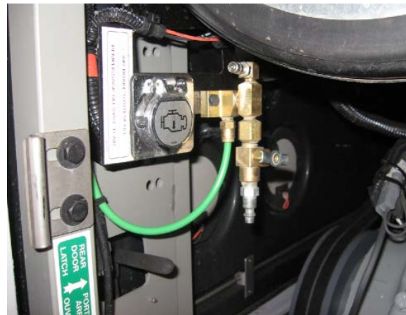
FIGURE 23 : ENGINE COMPARTMENT EMERGENCY AIR-FILL VALVE
