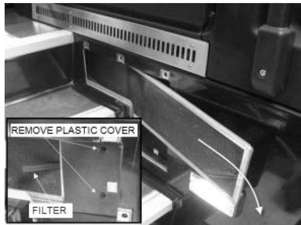
FIGURE 18: REMOVING DRIVER'S SECTION AIR FILTERS
