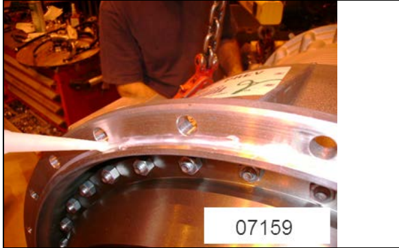
FIGURE 12: SILICONE APPLICATION TRANSMISSION HOUSING
