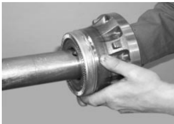
FIGURE 11: SLIP UNITIZED HUB BEARING OVER SPINDLE
