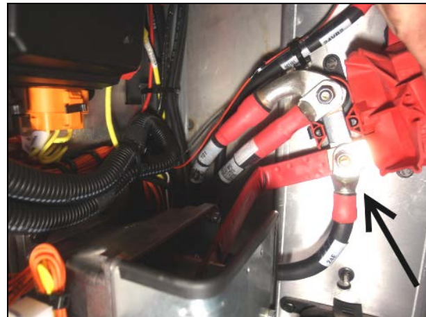
Figure 3: Bussman Junction Block - H3 Series.
