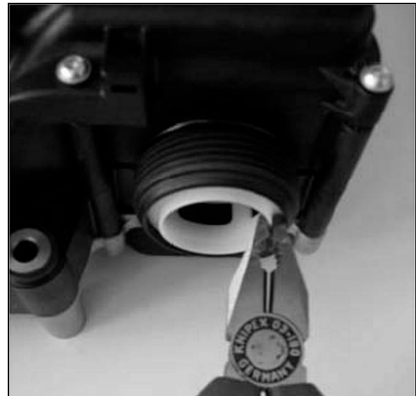
FIGURE 12 : PUMP ASSEMBLY FILTER ELEMENT
