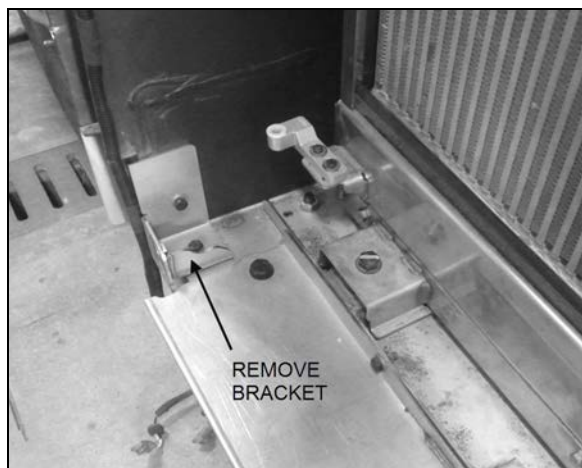
FIGURE 49: RADIATOR DOOR LOWER HINGE BRACKET
