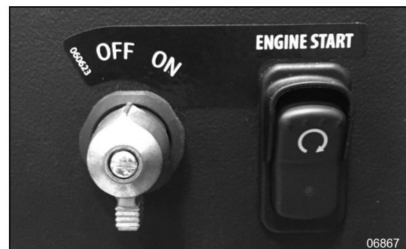
FIGURE 60: SWITCH ARRANGEMENT WITH STARTING MODULE
