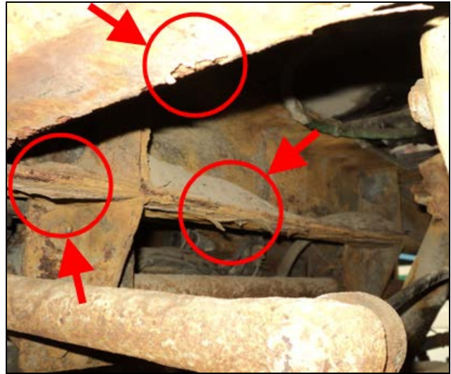
FIGURE 3: METAL FLAKING AND ACCUMULATED SAND
