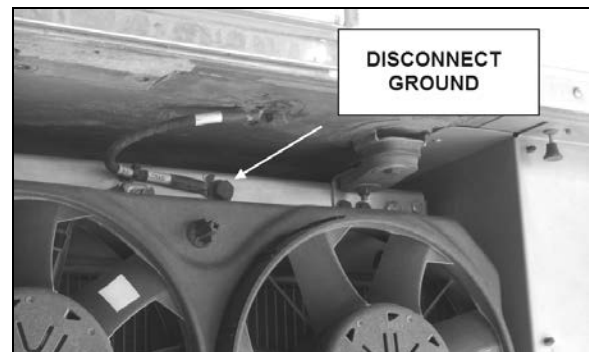
FIGURE 32: COOLING ASSEMBLY GROUND
