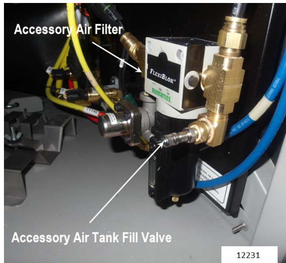
FIGURE 4: FRONT SERVICE COMPARTMENT
