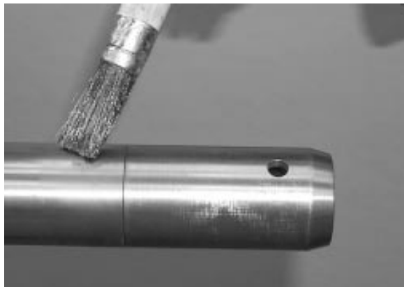
FIGURE 10: APPLY GLEITMO 805 GREASE
