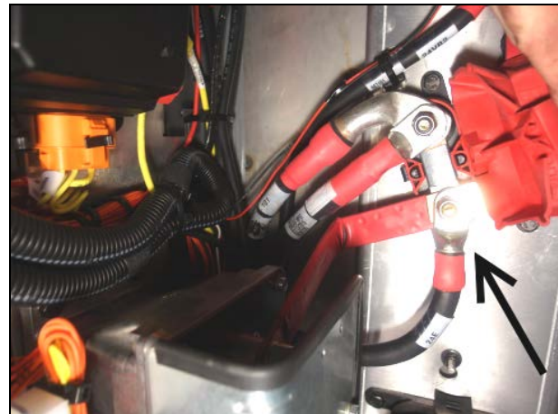
Figure 3: Bussman Junction Block - H3 Series.
