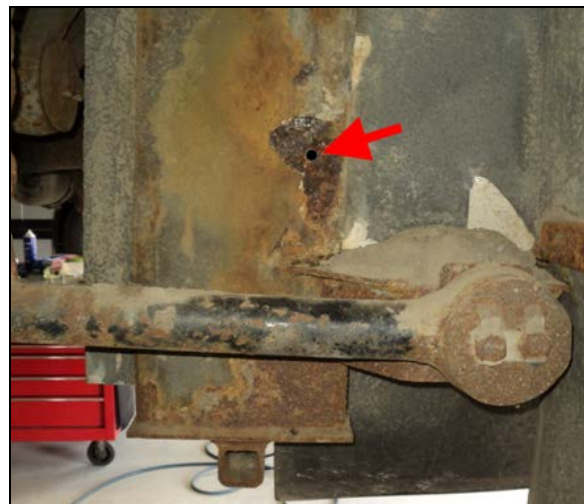
FIGURE 7: HOLE DRILLED IN STRUCTURAL MEMBER
