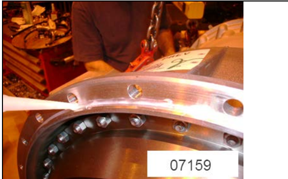
FIGURE 12: SILICONE APPLICATION TRANSMISSION HOUSING
