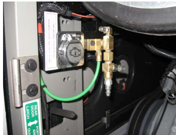
FIGURE 23 : ENGINE COMPARTMENT EMERGENCY AIR-FILL VALVE
