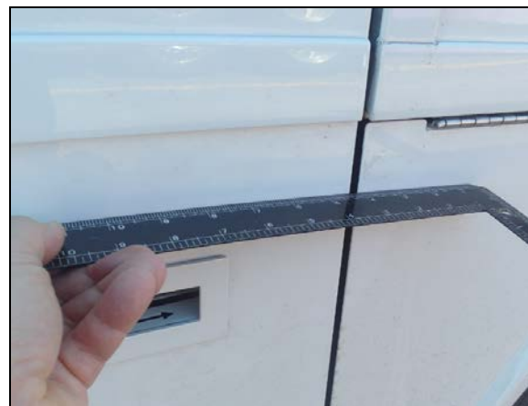
FIGURE 62: USE A RULER (SHOWN IN BLACK) TO CHECK THAT SURFACES ARE EVEN
