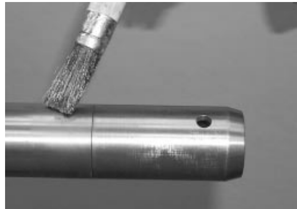
FIGURE 19: APPLY GLEITMO 805 GREASE
