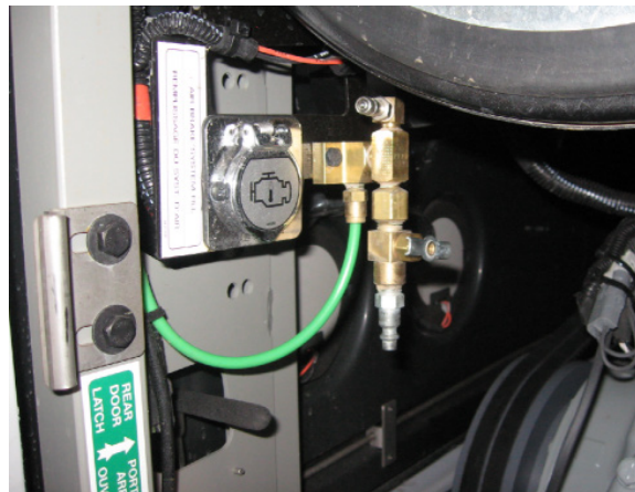
FIGURE 23 : ENGINE COMPARTMENT EMERGENCY AIR-FILL VALVE
