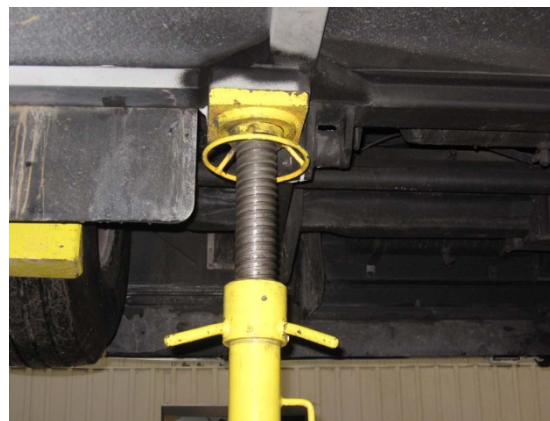
FIGURE 4 : JACK STAND AT CHASSIS HOISTING POINT - AFT OF FRONT AXLE (BOTH SIDES)
