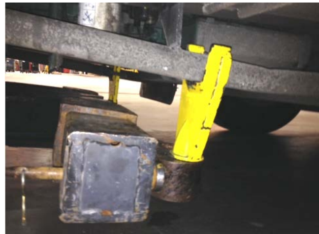
FIGURE 61 : PROPER LOCATION WHEN LIFTING THE SIDE MEMBERS
