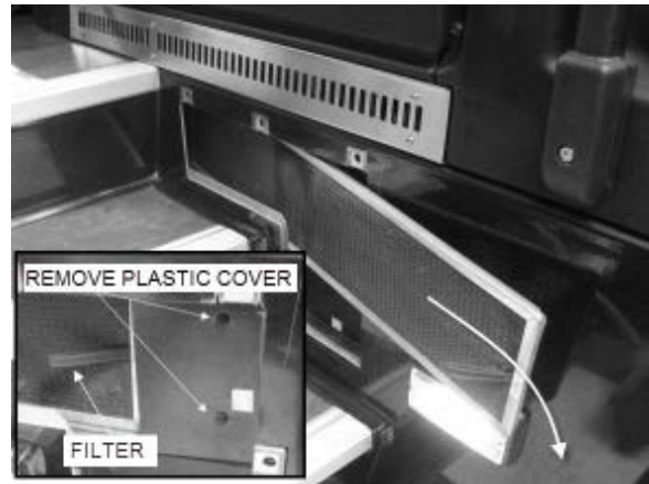
FIGURE 18: REMOVING DRIVER'S SECTION AIR FILTERS
