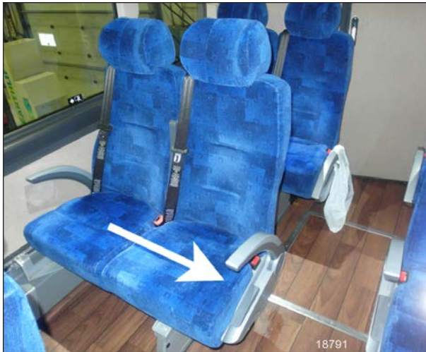
PULL TO UNLOCK THE ROTATION
