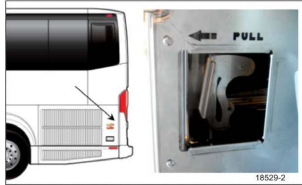
FIGURE 8: RADIATOR DOOR LATCH RELEASE LEVER LOCATION
