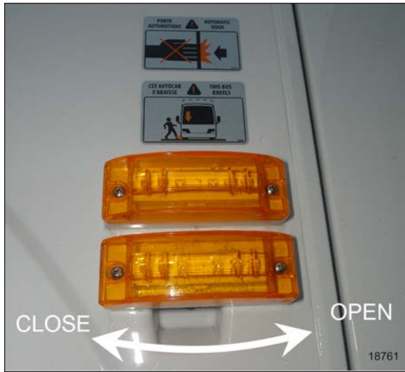
FIGURE 23: ENTRANCE DOOR EXTERIOR SWITCH – H3
