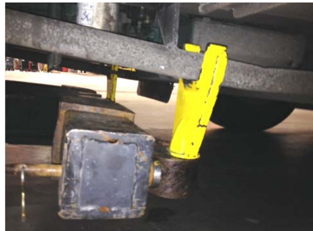
FIGURE 61 : PROPER LOCATION WHEN LIFTING THE SIDE MEMBERS
