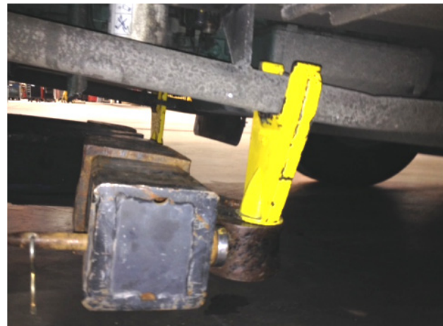
FIGURE 61 : PROPER LOCATION WHEN LIFTING THE SIDE MEMBERS
