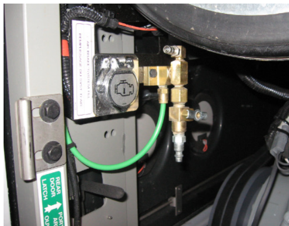
FIGURE 23 : ENGINE COMPARTMENT EMERGENCY AIR-FILL VALVE
