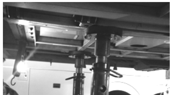
FIGURE 21: JACK STANDS UNDER THE FUEL TANK CRADLE
