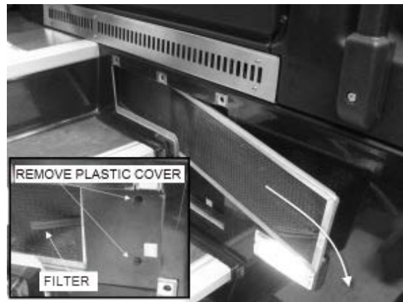
FIGURE 18: REMOVING DRIVER'S SECTION AIR FILTERS
