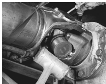
FIGURE 15: UNSEATING BEARING CUP ASSEMBLIES
