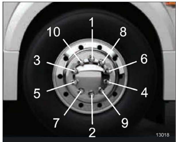
TIGHTENING SEQUENCE
