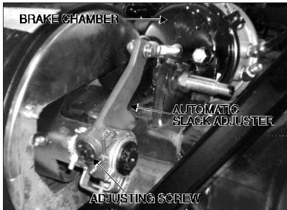
FIGURE 14: DRUM BRAKE ASSEMBLY 12044
