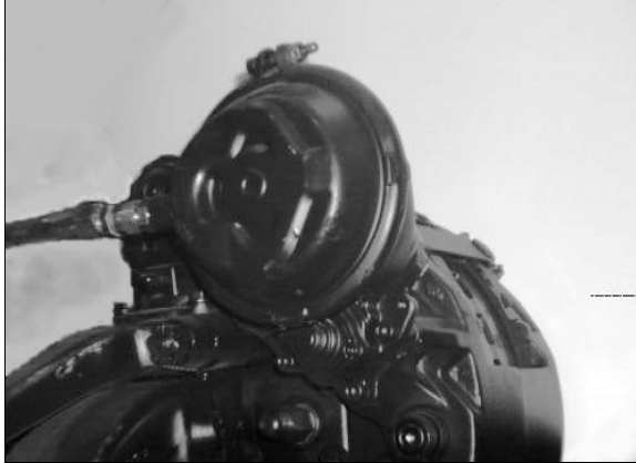
FIGURE 19: FRONT AXLE BRAKE AIR CHAMBER 12049
