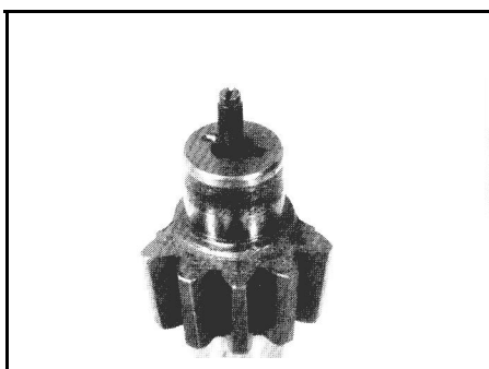
Inspect adjusting screw and retainer
