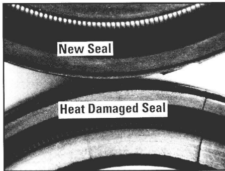
Inspect old seal
