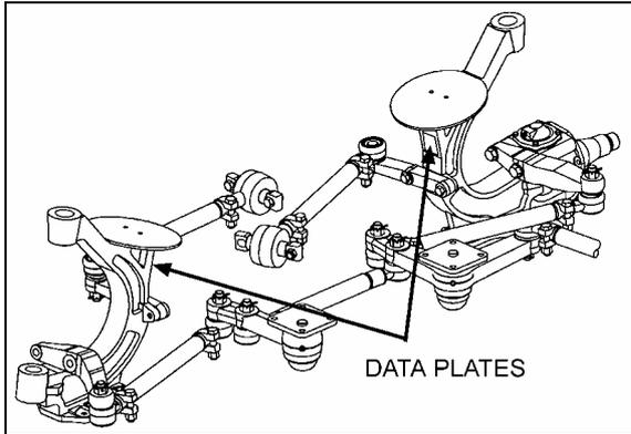
**FIGURE 7: ISS TYPICAL SERIAL & MODEL NUMBERS**00025C
