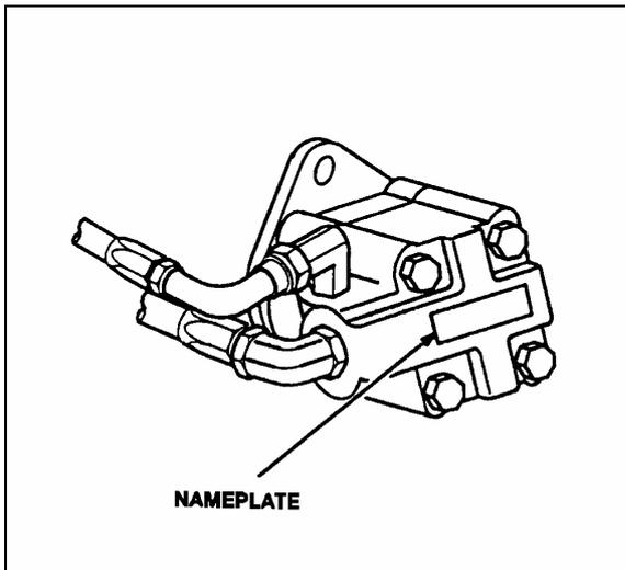
**FIGURE 8 : POWER STEERING PUMP SERIAL NUMBER** 00035
