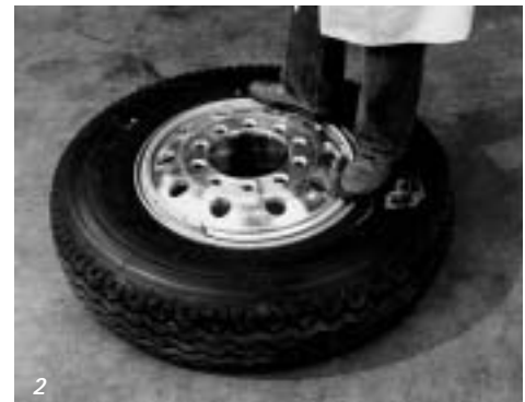
2 If the wheel requires a lock ring, start the leading edge of the lock ring being sure that it is seating in the machined groove. Then walk the lock ring onto the wheel, as illustrated
