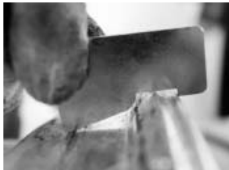
Photo 1. Acceptable Rim Flange Wear Condition
