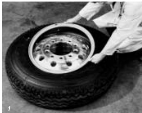
1 Lubricate tube, flap and wheel. Insert tube and flap into tire. Place them on the wheel so that the valve is aligned with the valve slot.
