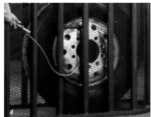
4 Inflate to 10 psi. Check to see that all components are properly in place. If not, deflate the tire by removing the valve core and reposition components properly. Place in a safety cage or other suitable restraining device (refer to OSHA rule 1910.177, paragraph B, see Section 7, page 44). Use clip-on chuck and stand behind barrier during inflation. Do not lean on cage. Inflate to recommended pressure. Deflate completely to avoid localized over-stretching of the tube. Reinflate to the tire manufacturer's recommended pressure.
