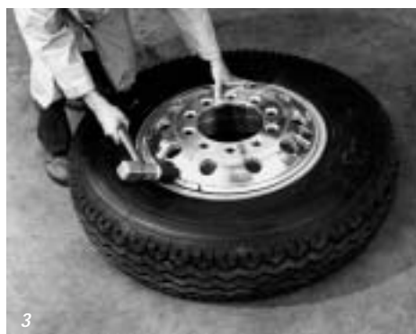
3 Seat the second end of the split side ring or lock ring with a rubber, plastic or leather-facet mallet as shown. Check carefully to see that the split side ring or side ring and lock ring assembly is in the proper position. If not, completely remove the components and start over.
