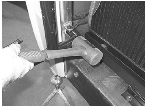
FIGURE 64: PANTOGRAPH ARM ADJUSTMENT
