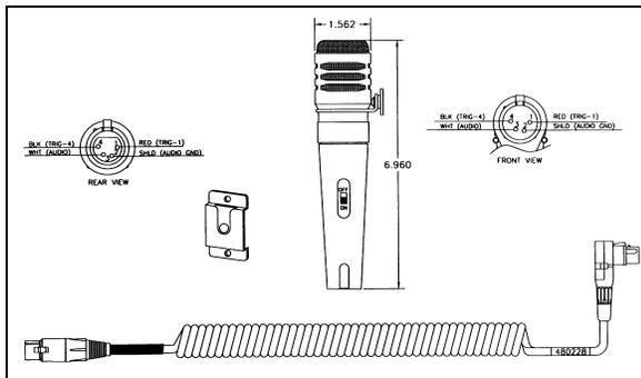
FIGURE 11: RUBBER COATED MICROPHONE 23217
