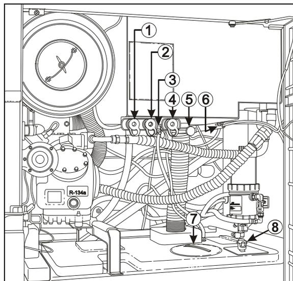
FIGURE 27: F/W TANK SERVICE VALVES
