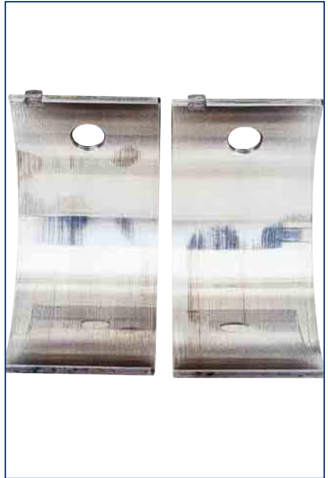
Cam bearings show minor polishing.
