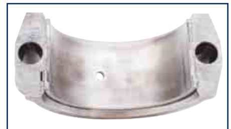
Rod bearings show only minor overlay wear.
