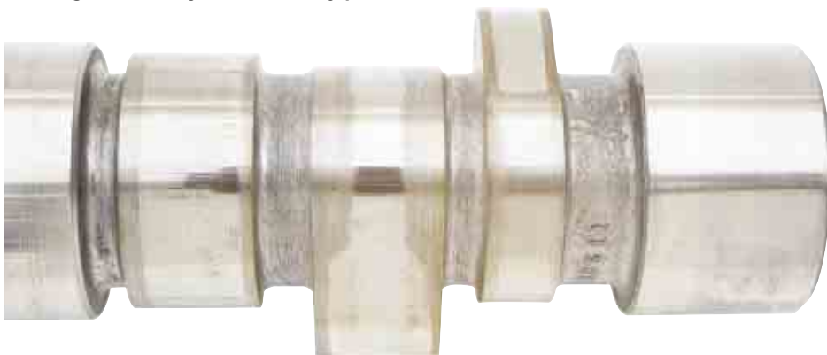
Camshaft looks excellent. Journals and lobes show only contact path polishing.
