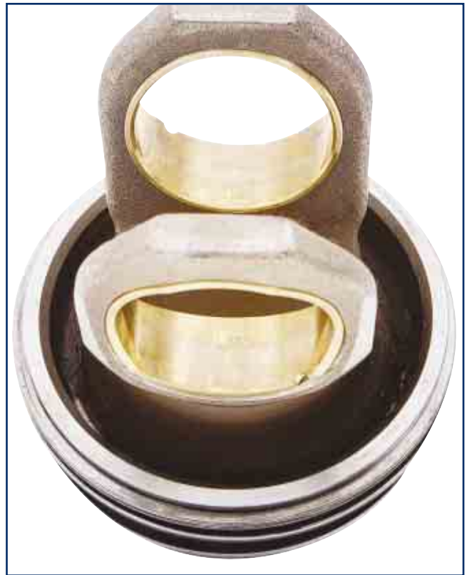
Piston bushings only show typical polishing.
