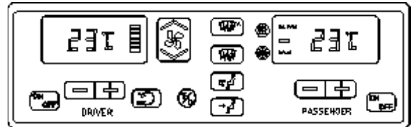
FIGURE 5: CENTRAL HVAC SYSTEM CONTROL UNIT 22296
