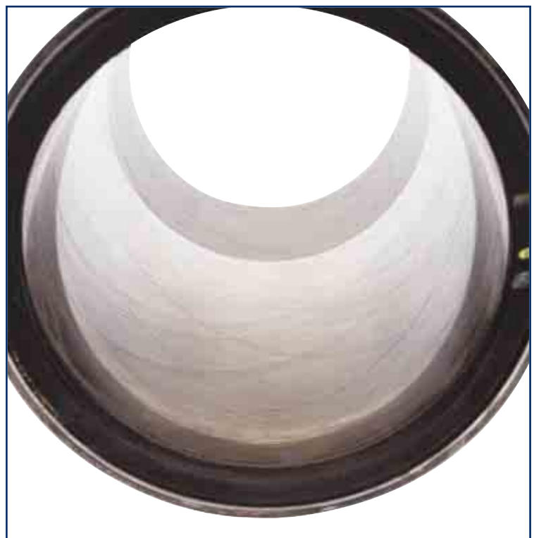
Piston liner shows cross hatch pattern intact.
