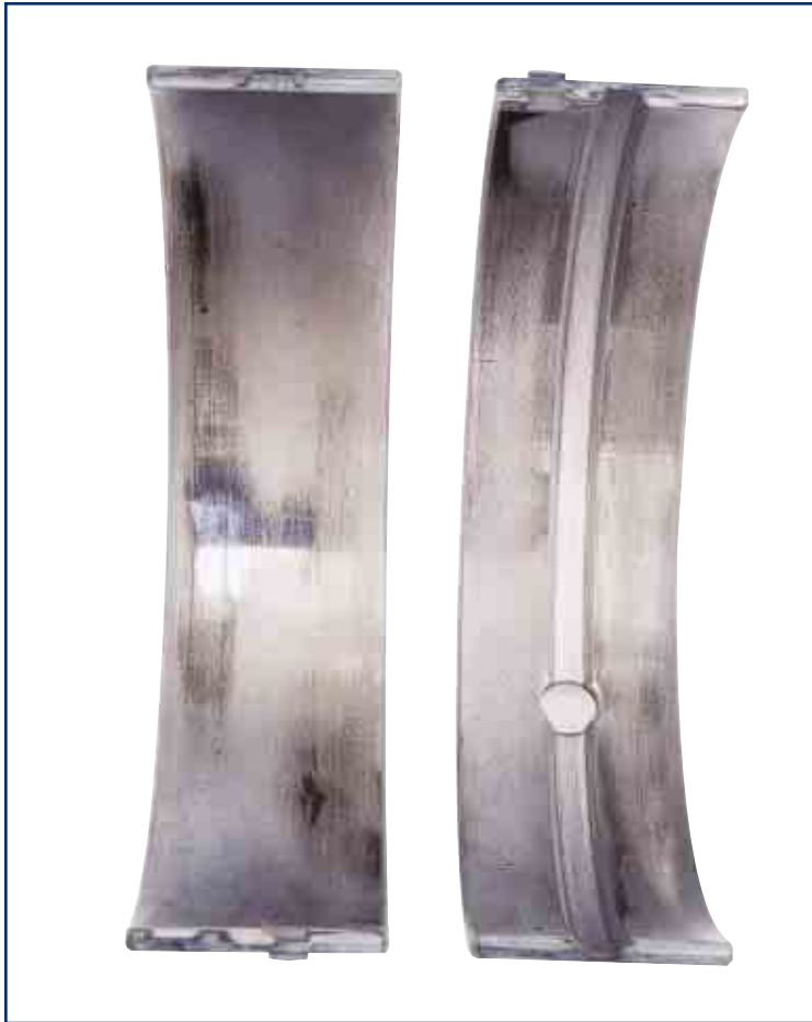
Main bearings did their job and show no wear. Upper no load main bearings show no wear and lower load bearings look as good. Bearings show only minor overlay polish.
