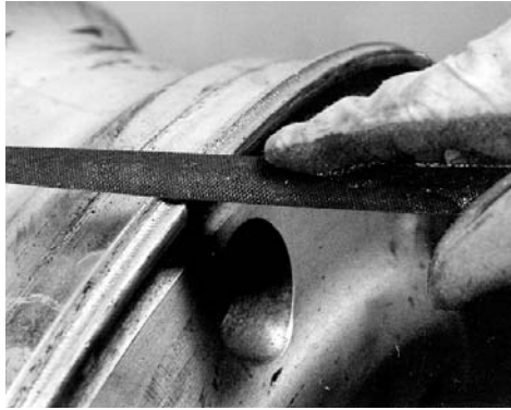
Photo 4. Removing sharp edge by hand with a metal file.
