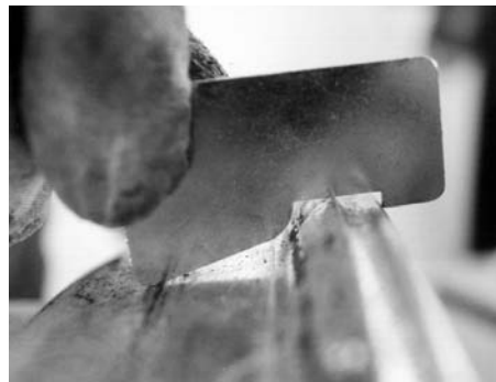
Photo 1. Acceptable Rim Flange Wear Condition
