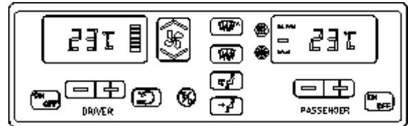
FIGURE 5: CENTRAL HVAC SYSTEM CONTROL UNIT 22296
