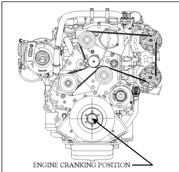
FIGURE 10: ENGINE CRANKING POSITION
