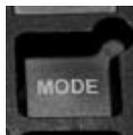
The TCM may automatically delete a code from memory if it has not recurred. If the MODE INDICATOR (LED) is not illuminated, the displayed code is not active. An illuminated MODE INDICATOR (LED) during normal operation signifies secondary shift mode operation.
