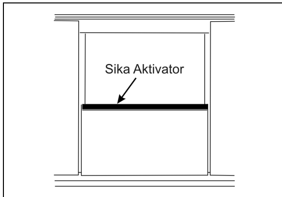
FIGURE 72 : SLIDING WINDOW - SIKa AKTIVATOR
