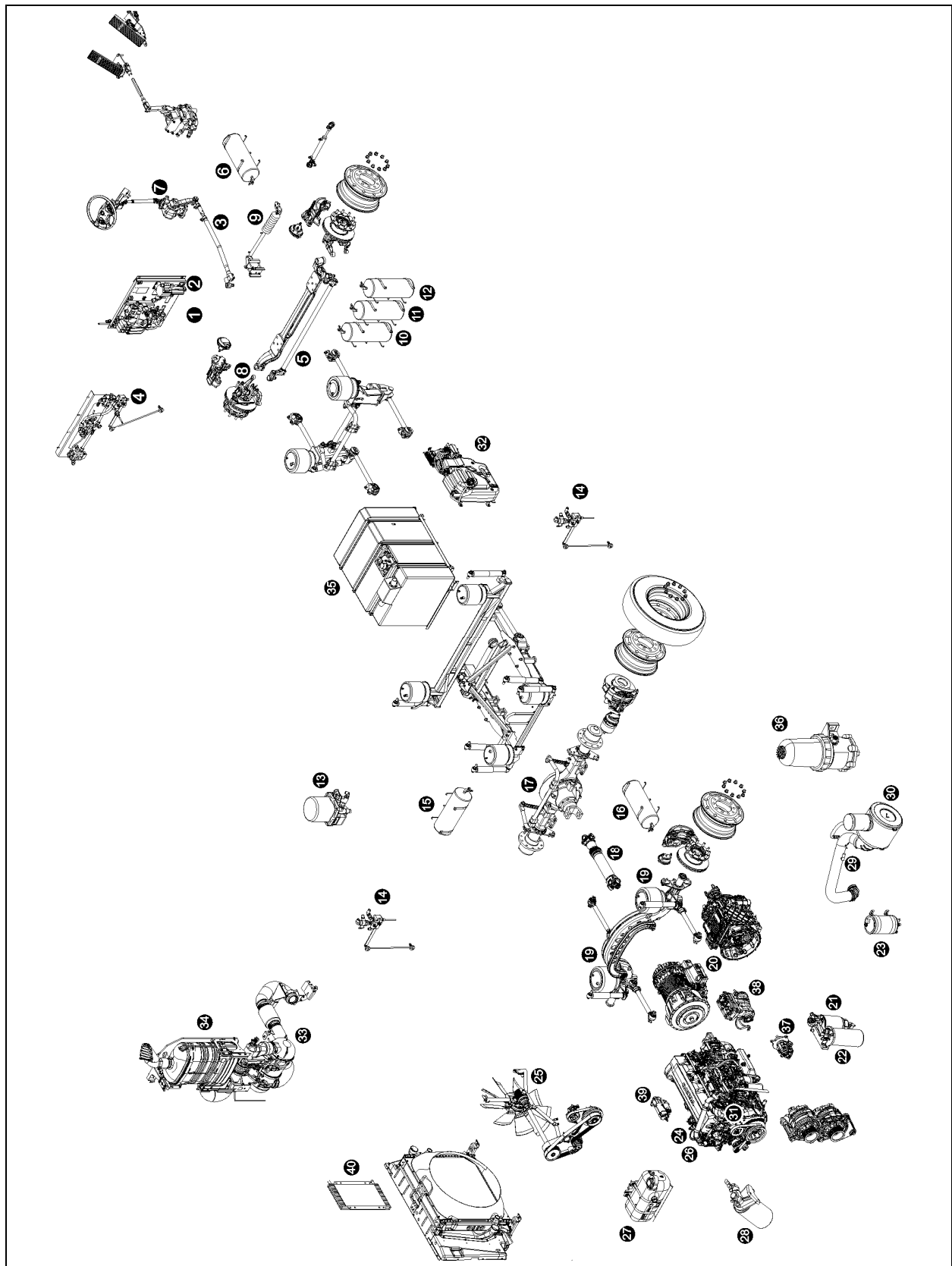
FIGURE 1: LUBRICATION AND SERVICING POINTS ON H3 SERIES VEHICLES (TYPICAL)
