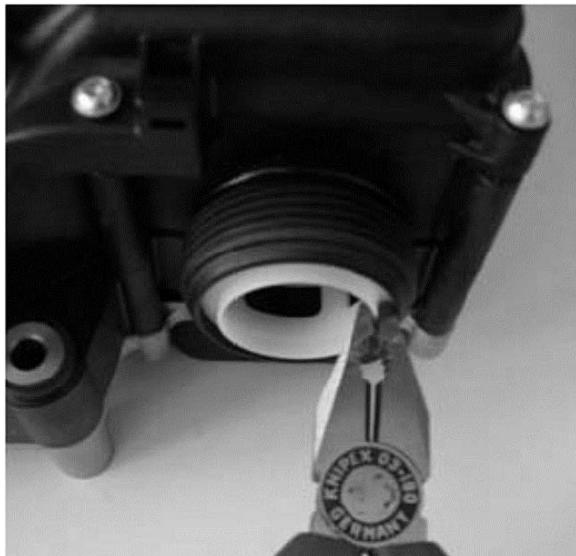
FIGURE 11 : PUMP ASSEMBLY FILTER ELEMENT
