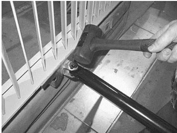
FIGURE 64: DOOR LATERAL ADJUSTMENT
