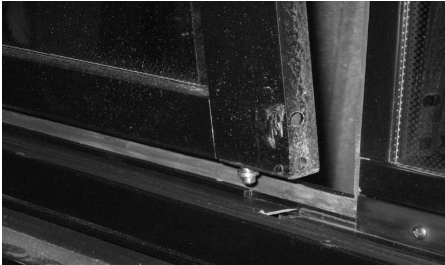
FIGURE 42: DISENGAGING THE BOTTOM OF THE SASH
