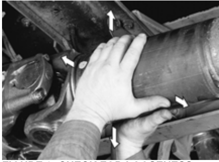
FIGURE 6: CHECK FOR LOOSENESS
