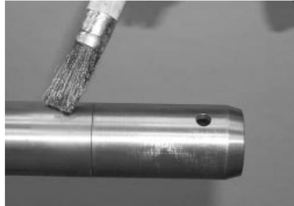
FIGURE 18: APPLY GLEITMO 805 GREASE
