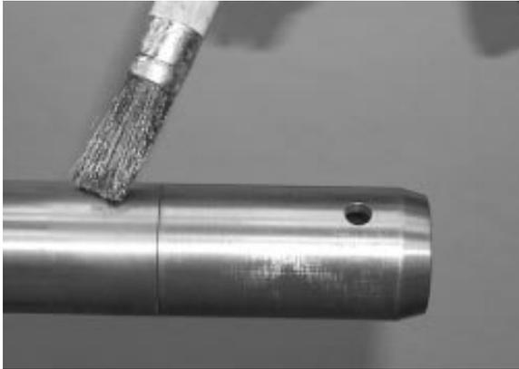
FIGURE 9: APPLY GLEITMO 805 GREASE
