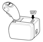
Continued descriptions in this instruction are based on "Gear selector Professional". All information is also relevant for "Gear selector Standard" except that describing +/- and E/P buttons
