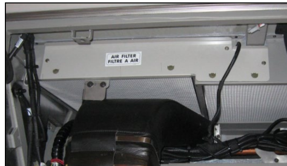
PASSENGERS AREA AIR FILTER REMOVAL
