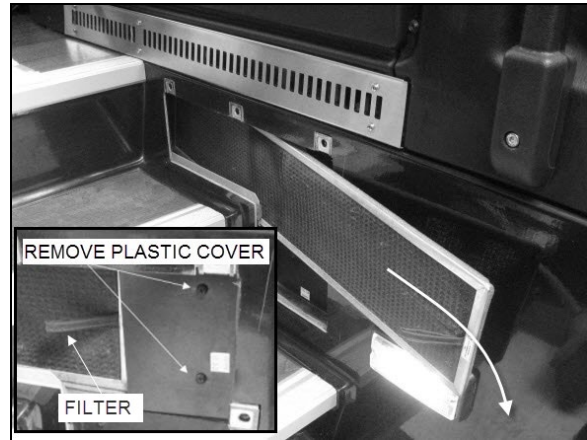
REMOVING DRIVER'S SECTION AIR FILTER
