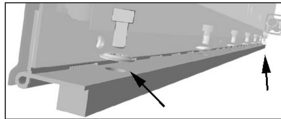
2. Close door and adjust in opening. A 1mm maximum difference between left and right measured gap is accepted.
