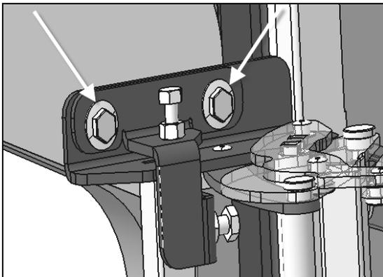
3. Using the top adjusting screws, adjust door to get a 6mm gap at the top.
