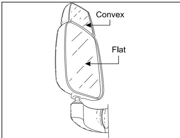
FIGURE 56: REAR VIEW MIRROR (RAMCO)
