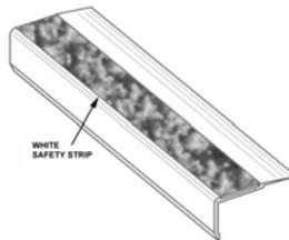
10. Temporarily fix white safety strip with a piece of duct tape, leaving 1 to 2 inches free at each end.
