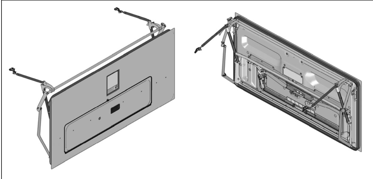
For the removal and installation of a wheelchair lift (WCL) cassette compartment door body panel, you will need:
