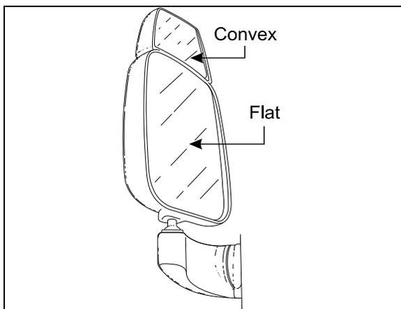
FIGURE 14: REAR VIEW MIRROR (RAMCO)
