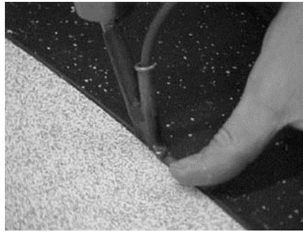
4. Always add an extra inch of filler bead at the beginning and at the end of repair.
