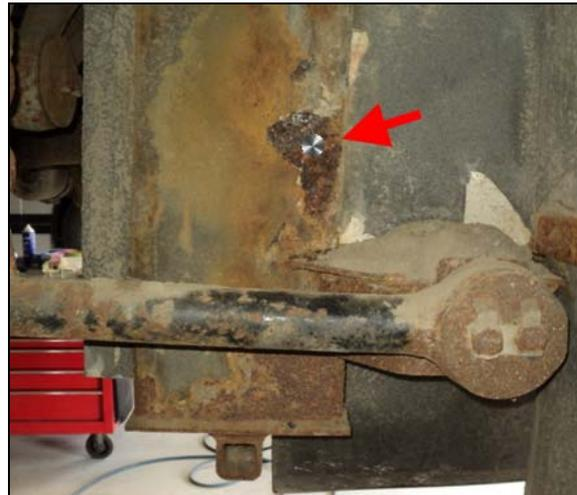
FIGURE 6: CLEANED SPOT ON STRUCTURAL MEMBER
