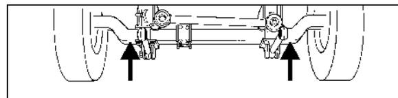
FIGURE 92: JACKING POINTS ON I-BEAM FRONT AXLE
