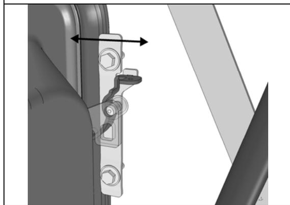
15. Check handle adjustment. Handle must remain tight against its plastic housing.
