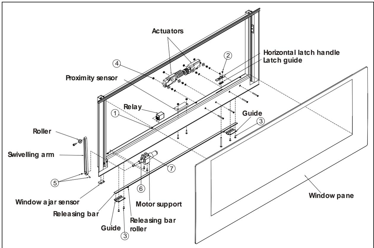
FIGURE 62: ELECTRIC AWNING WINDOW EXPLODED VIEW (SASH)
