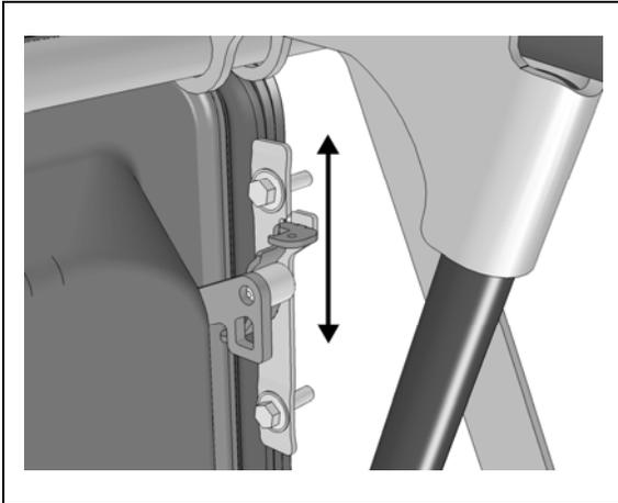
6. Open baggage compartment door and adjust using the cylinder mounting block.
