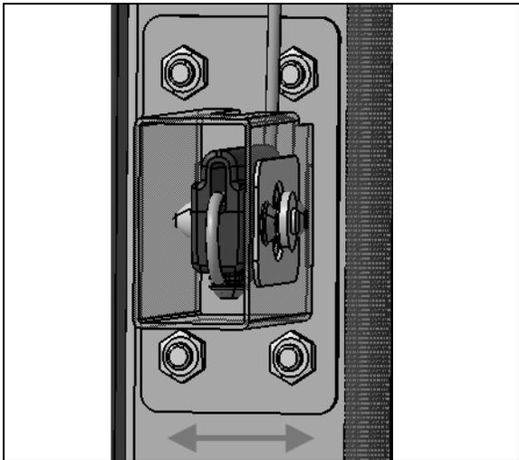
12. Make sure that backing plate is parallel to structure before tightening hardware
