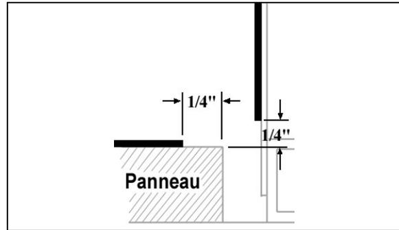
In the case of front finishing joint, apply some masking tape on each side of joint.
