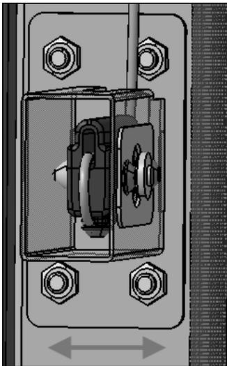
12. Make sure that backing plate is parallel to structure before tightening the retainer support hardware
