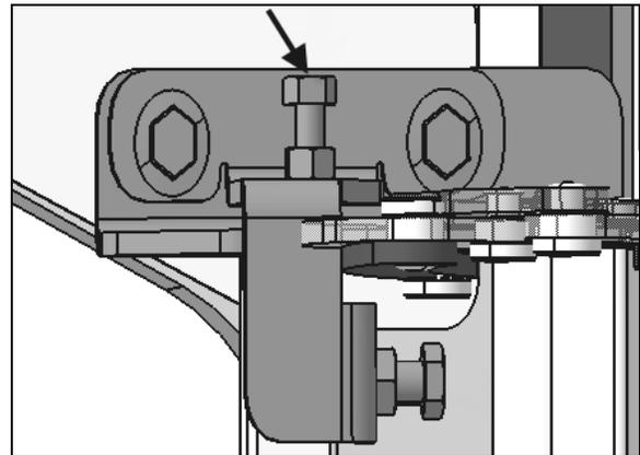
4. Using the 2 side adjusting screws (top and bottom), adjust door to get a 6mm to 8mm lateral gap (gap must be equal on both side).
