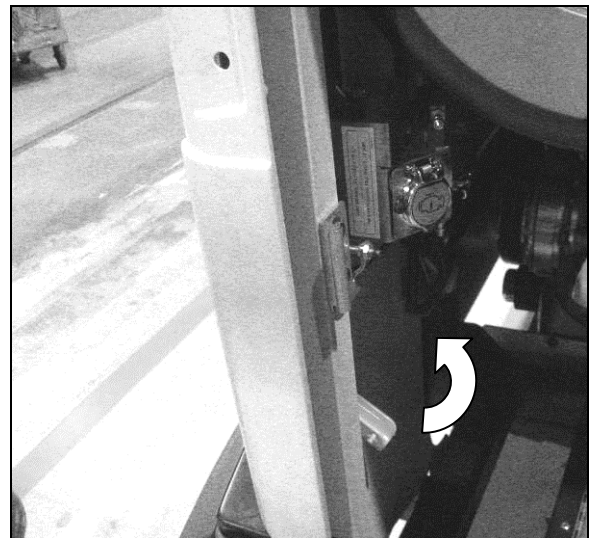
OPENING ENGINE COMPARTMENT REAR DOOR
