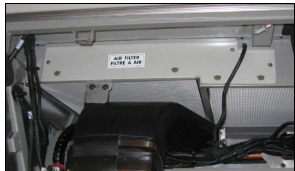
PASSENGERS AREA AIR FILTER REMOVAL
