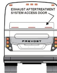
The engine door must be open before opening the exhaust aftertreatment system access door. To open the access door, lower the latch release lever, using a flat tip screwdriver.
