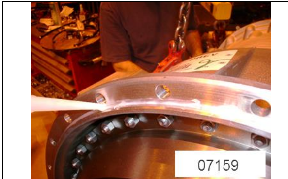
FIGURE 12: SILICONE APPLICATION TRANSMISSION HOUSING
