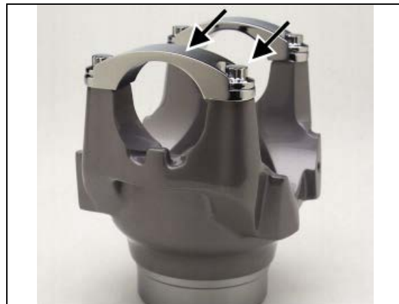
FIGURE 3: COLD FORMED BEARING RETAINER AND BOLTS AS USED ON PREVOST VEHICLES
