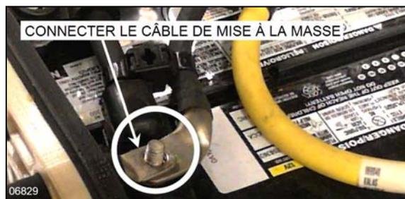
FIGURE 42: CÂBLE DE MISE À LA MASSE
