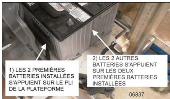
FIGURE 38: POSITION ADÉQUATE DES BATTERIES
