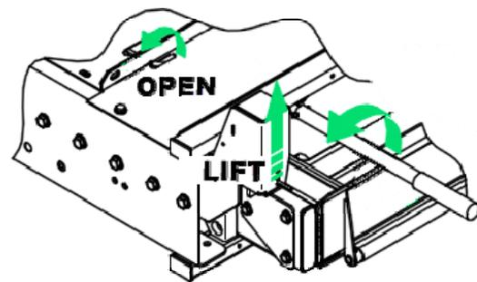
4. Grasp the platform and pull firmly until the lift is all the way out against the carriage stops.
