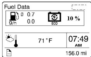
When equipped with PRIME option, the percentage of trip made on regenerated electricity is also displayed.
