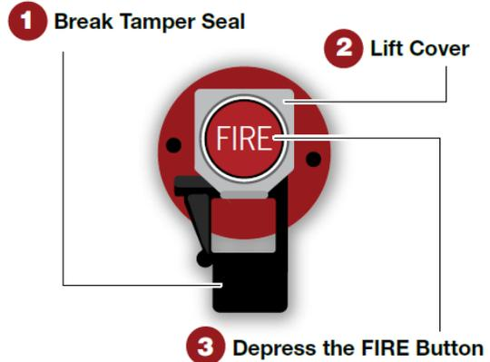
**CAUTION:** The extinguisher discharge may cause an obscuring cloud behind and near the vehicle.
