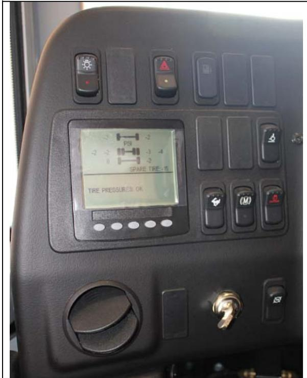
The L.H. dashboard panel includes controls for the operation of the coach; it also includes the ignition switch and an adjustable air vent.
