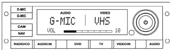
The VSS-05 Video and Sound Selector enables the driver to select audio, audio/video and video source with settings of volume level, bass, treble, etc. for the passenger's area only. The
