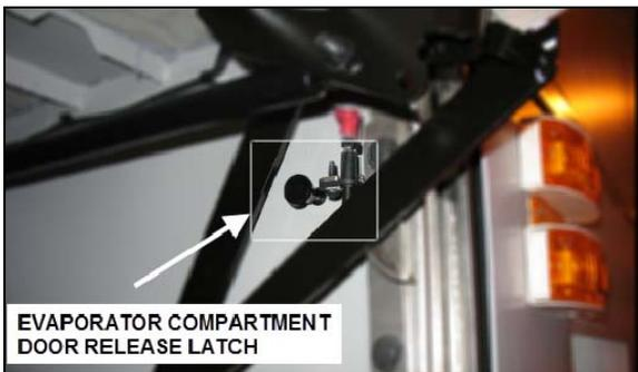
EVAPORATOR COMPARTMENT DOOR RELEASE LATCH
