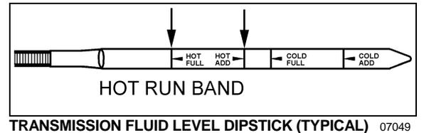
Replace dipstick and tighten the filler tube cap until the rubber seal is correctly seated.
