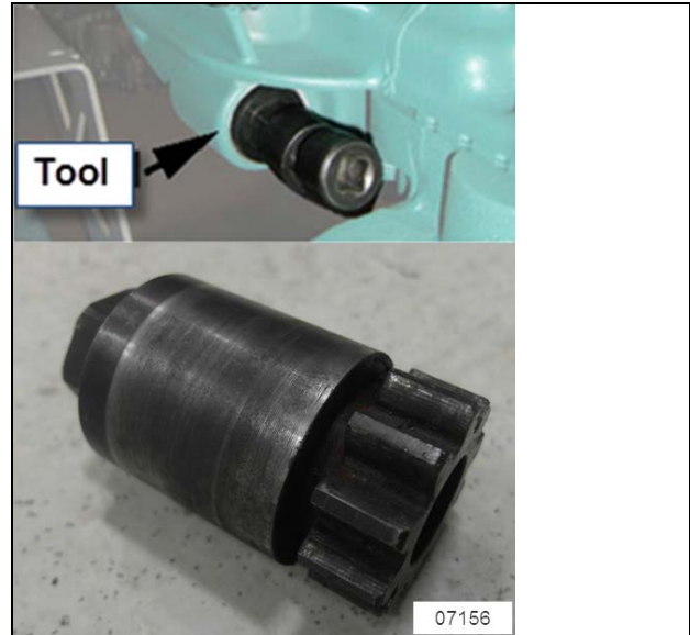
FIGURE 10: VOLVO ENGINE TURNING TOOL #88800014
