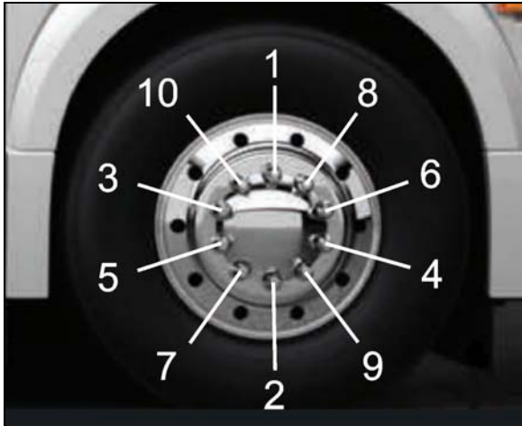
TIGHTENING SEQUENCE
