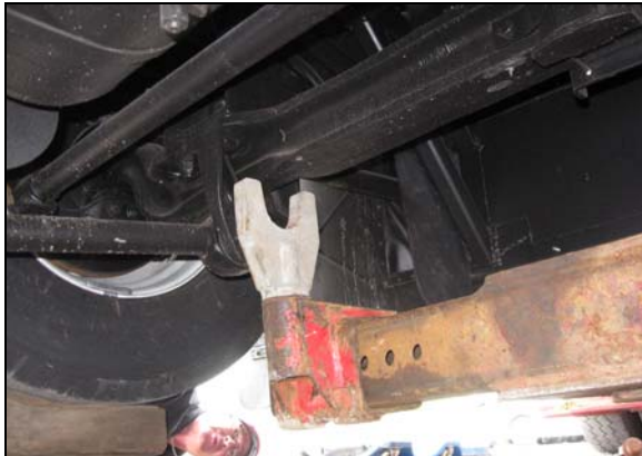
LIFTING FROM UNDER THE FRONT AXLE
