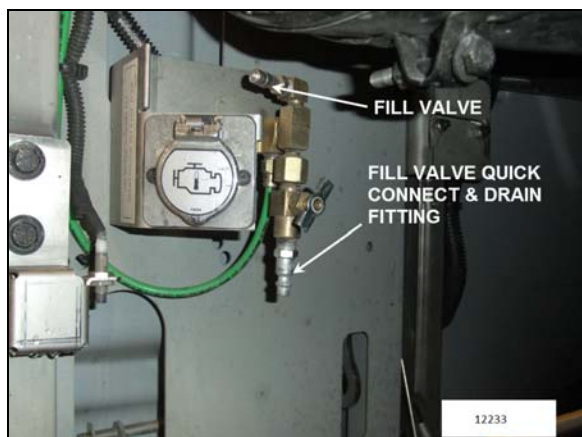
FIGURE 6: REAR VALVE LOCATION (TYPICAL)
