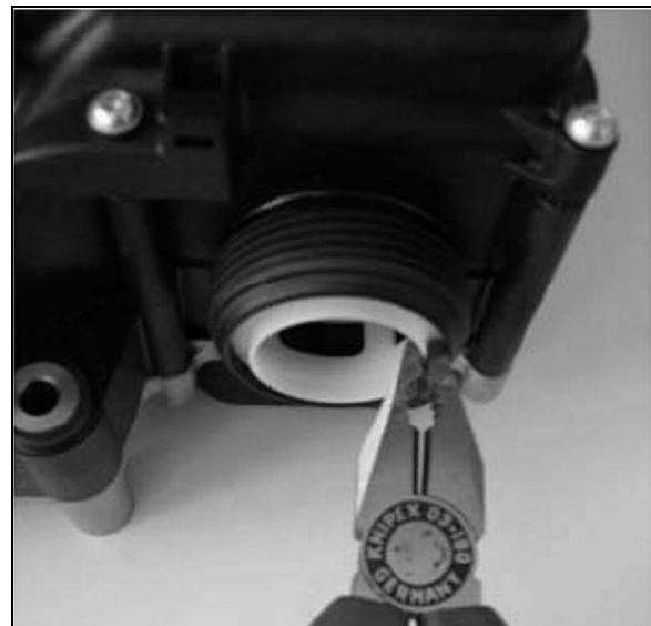
FIGURE 12 : PUMP ASSEMBLY FILTER ELEMENT
