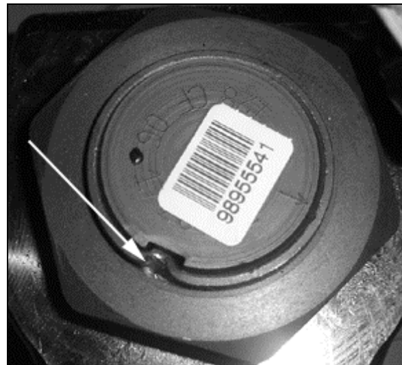
FIGURE 20: FIXING NUT PUNCH MARK
