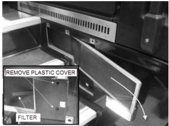
FIGURE 18: REMOVING DRIVER'S SECTION AIR FILTERS
