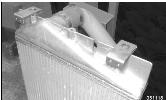
FIGURE 41: CAC UPPER BRACKETS & PIPE
