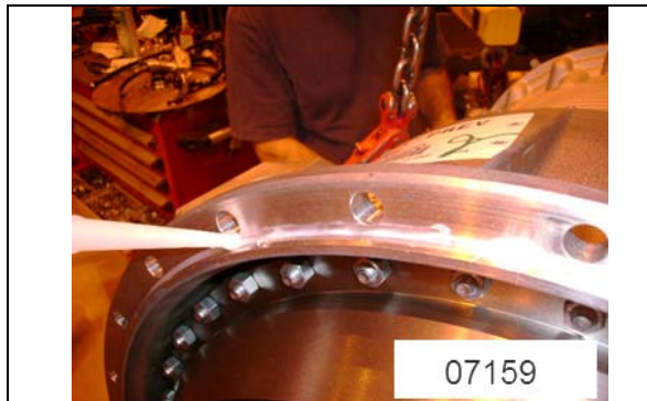
FIGURE 12: SILICONE APPLICATION TRANSMISSION HOUSING
