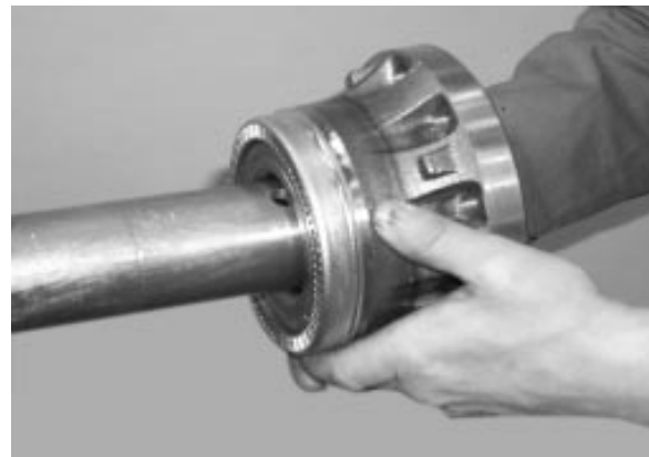
FIGURE 20: SLIDE UNITIZED HUB BEARING OVER SPINDLE
