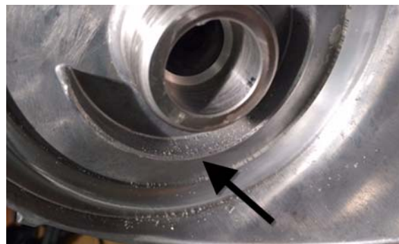
ALUMINUM PARTICLES ON THE FILTER RESTRICTOR (FUEL FILTER HOUSING)
