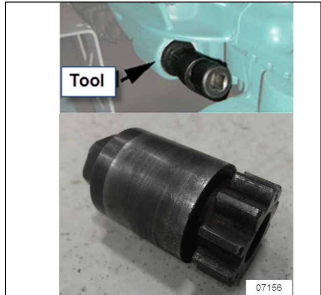
FIGURE 10: VOLVO ENGINE TURNING TOOL #88800014
