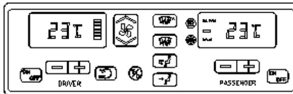
CENTRAL HVAC SYSTEM CONTROL MODULE 22296
