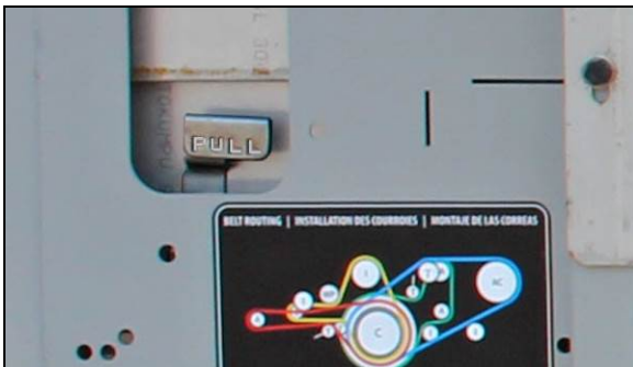
RADIATOR DOOR RELEASE HANDLE
