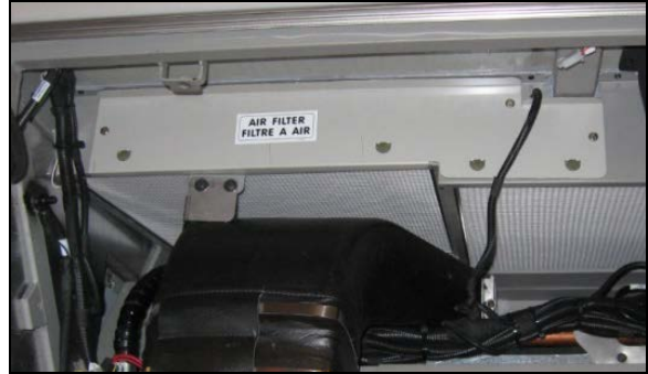
PASSENGERS AREA AIR FILTER REMOVAL 22306
