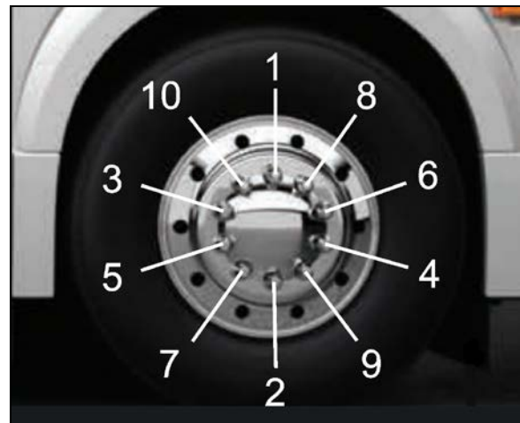
TIGHTENING SEQUENCE
