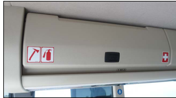
A DECAL INDICATES THAT A FIRE HATCHET, A FIRE EXTINGUISHER AND A FIRST-AID KIT ARE LOCATED IN THIS OVERHEAD COMPARTMENT
