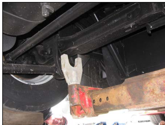
LIFTING FROM UNDER THE FRONT AXLE
