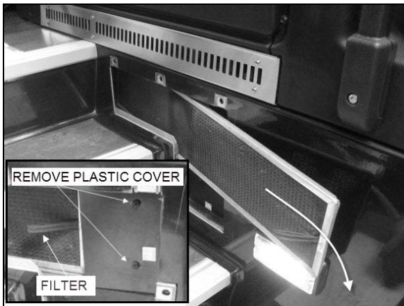
REMOVING DRIVER'S SECTION AIR FILTER
