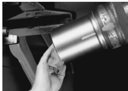
FIGURE 24: CLEAN GREASE FROM SPLINE SLEEVE
