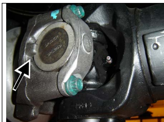
FIGURE 28: YOKE TAB (EAR)
