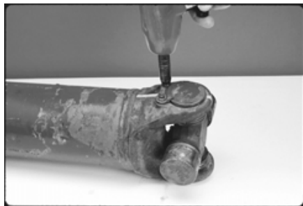
FIGURE 17: SPRING TAB BOLTS REMOVAL
