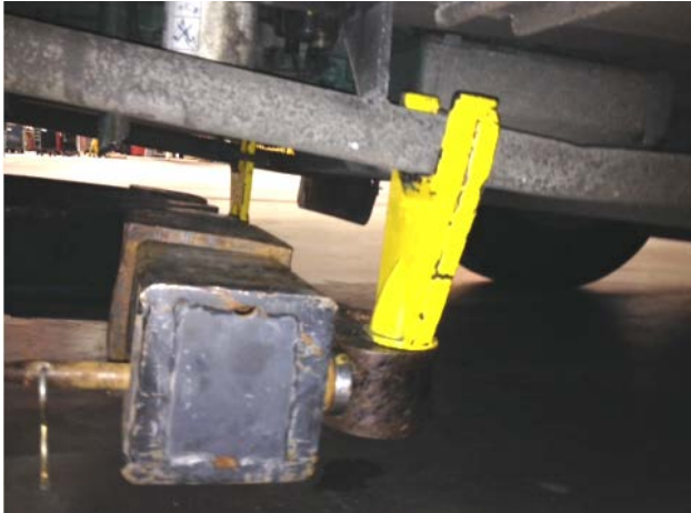
FIGURE 61 : PROPER LOCATION WHEN LIFTING THE SIDE MEMBERS
