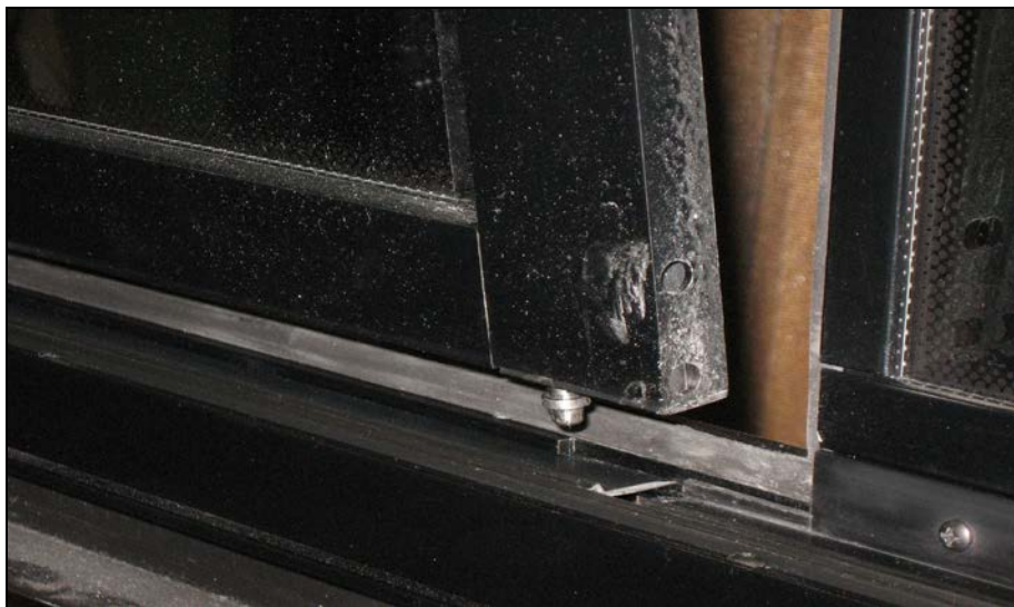
FIGURE 101: DISENGAGING THE BOTTOM OF THE SASH
