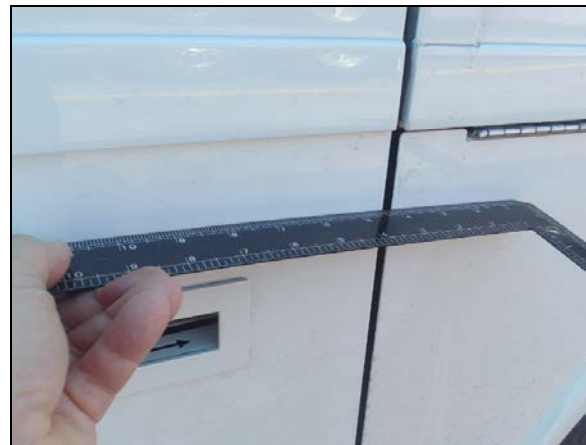
FIGURE 62: USE A RULER (SHOWN IN BLACK) TO CHECK THAT SURFACES ARE EVEN
