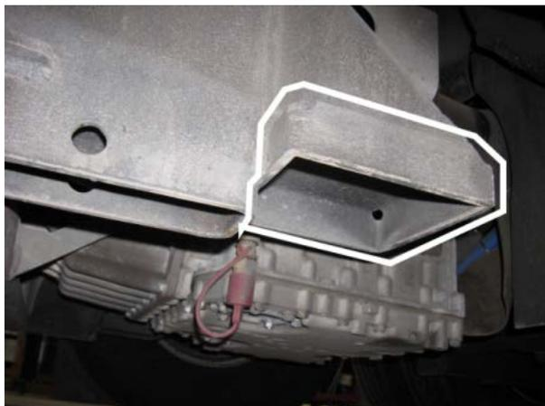
**FIGURE 15: SUPPORT DE LEVAGE AU CHÂSSIS
