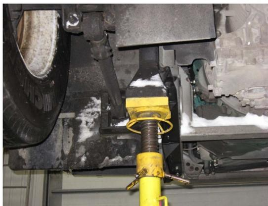
**FIGURE 20: CHANDELLE AU SUPPORT DE LEVAGE -
