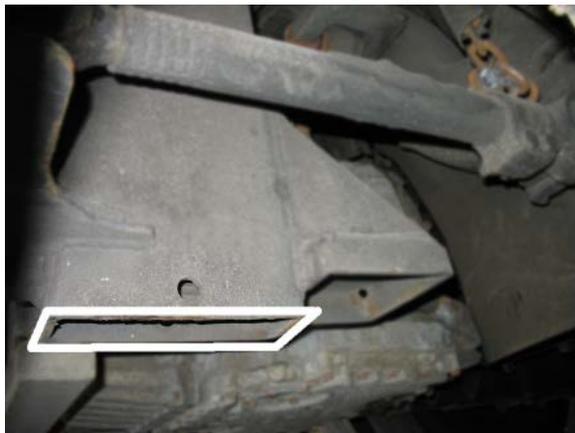
FIGURE 3: POINTS DE LEVAGE DU CHÂSSIS
