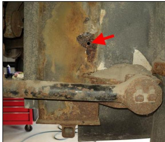
FIGURE 7: TROU PERCÉ DANS LE CHÂSSIS
