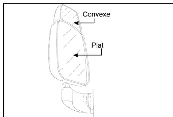
FIGURE 92 : RÉTROVISEUR (RAMCO)
