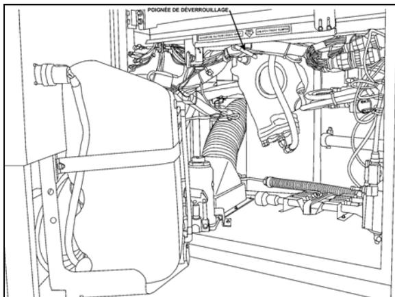
FIGURE 12: POIGNÉE DE DÉVERROUILLAGE DU PARE-CHOC AVANT 18613
