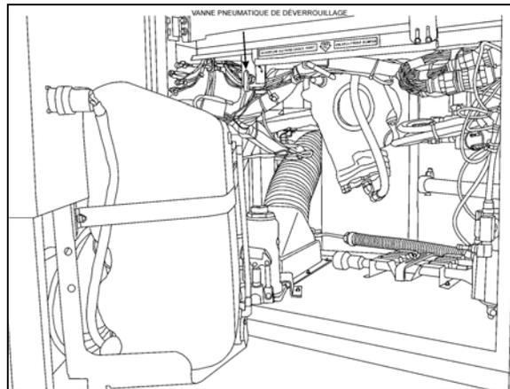
FIGURE 26: SOUPAPE D'OUVERTURE D'URGENCE EXTÉRIEURE 12209
