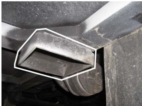
**FIGURE 16: SUPPORT DE LEVAGE AU CHÂSSIS
