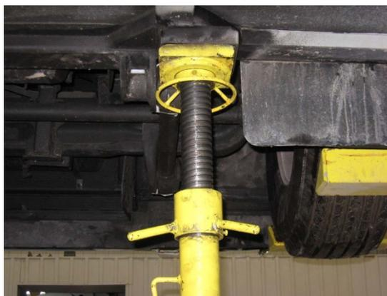
**FIGURE 18: CHANDELLE AU SUPPORT DE LEVAGE -
