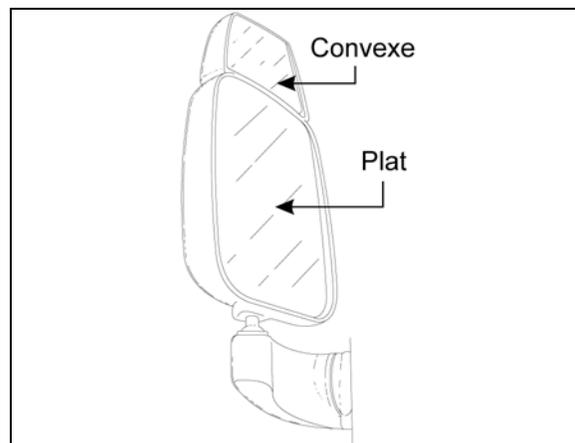
FIGURE 15 : RÉTROVISEUR (RAMCO)
