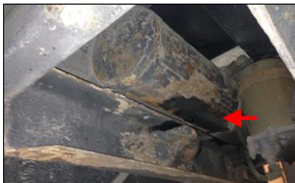
FIGURE 9: APPLICATION DE TECTYL 185GW BLACK
