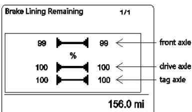
The numerical values indicate the brake lining remaining in 1/32 inch, mm or in term of percentage (%), depending on the unit selected in Display Settings menu (new brake pads are displayed as 100% if the unit selected is %).
