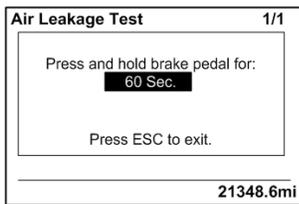
g. You must press and hold brake pedal for 60 seconds, as instructed.
