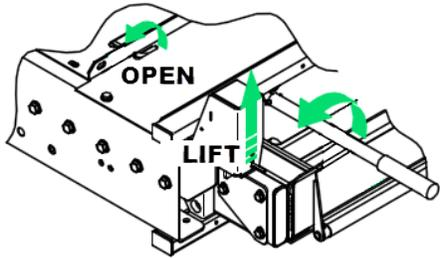
5. Grasp the top edge of the front rolls top with two hands and pull firmly. The platform moves smoothly after an initial resistance. Pull platform straight out to the end of its travel.
