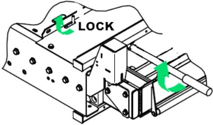
6. Lift right handrail to the vertical and push firmly down into its socket. Repeat for left handrail.
