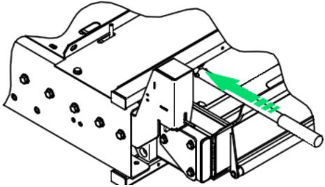
4. Rotate the keyed release shaft 1/4-turn (as indicated on the adjacent decal) while lifting stow lock lever simultaneously.
