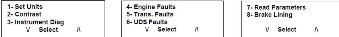
This menu exits to the drive mode screen when there has been inactivity for 5 seconds.
