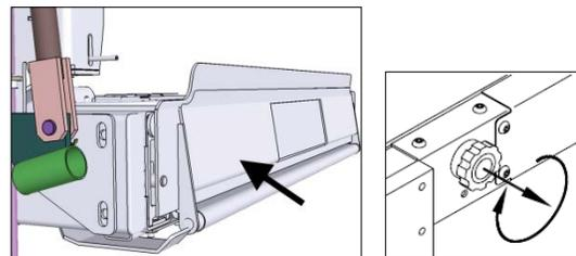
4. Lift the left handrail upward out of its socket. Lower handrail to the platform. Repeat for the right handrail.
