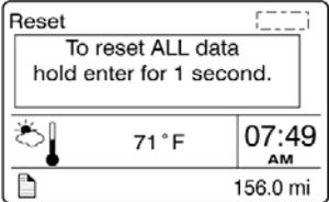
When the Reset Trip Data menu is open, pressing and holding down the ENTER button for more than 1 second resets the functions listed below. This function will permit to the system to calculate new value from the point of resetting.
