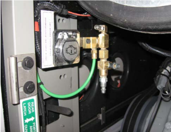
FIGURE 23 : ENGINE COMPARTMENT EMERGENCY AIR-FILL VALVE
