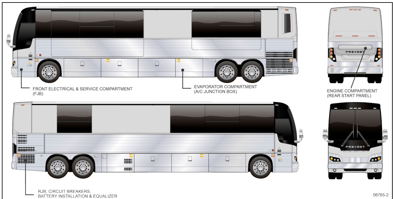
FIGURE 14: ELECTRICAL COMPARTMENTS (X3-45 VIP)
