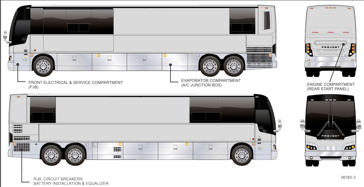
FIGURE 15: ELECTRICAL COMPARTMENTS (X3-45 VIP COMMERCIAL BUS SHELL)
