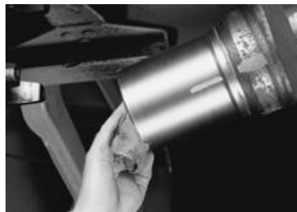
FIGURE 24: CLEAN GREASE FROM SPLINE SLEEVE
