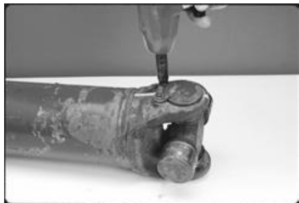
FIGURE 17: SPRING TAB BOLTS REMOVAL
