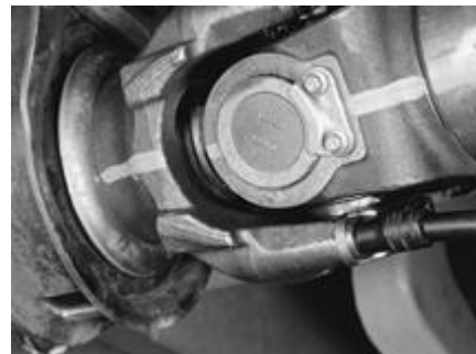
FIGURE 27: ALIGN THE PHASING MARKS BETWEEN THE YOKE AND PROPELLER SHAFT
