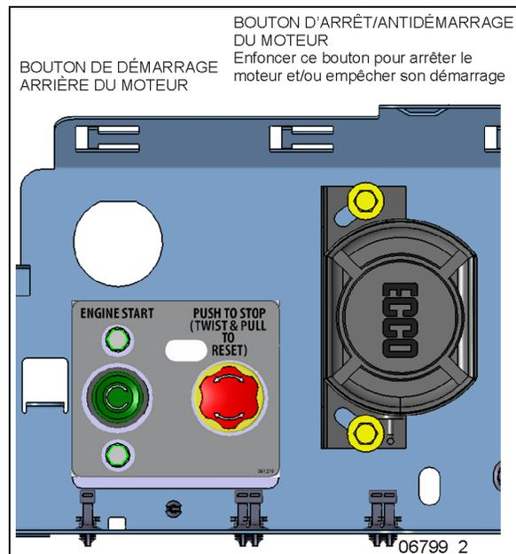
FIGURE 30: SÉRIE H3 — PANNEAU DE DÉMARRAGE ARRIÈRE
