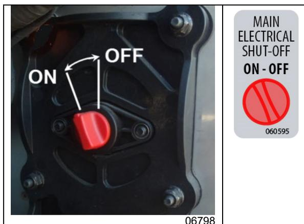
FIGURE 40 : INTERRUPTEUR PRINCIPAL D'ALIMENTATION – SÉRIE X3
