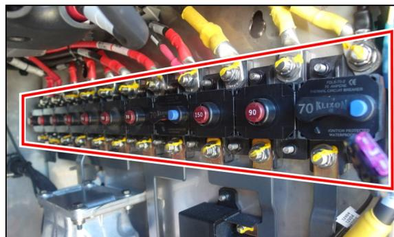
FIGURE 20: DISJONCTEURS PRINCIPAUX DANS LE COMPARTIMENT PRINCIPAL D'ALIMENTATION
