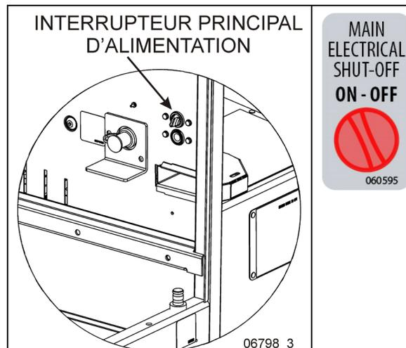
FIGURE 41: INTERRUPTEUR PRINCIPAL D'ALIMENTATION – SÉRIE H3
