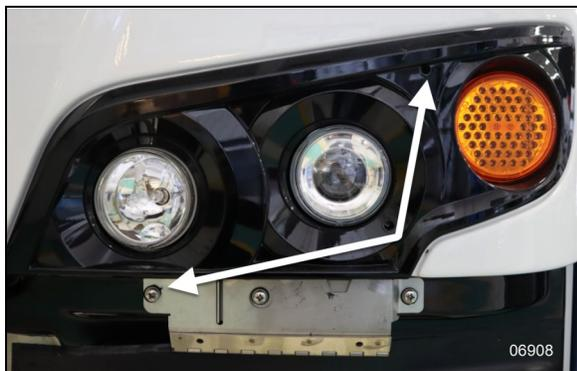
FIGURE 71: HEADLAMPS ASSEMBLY FIXING SCREWS
