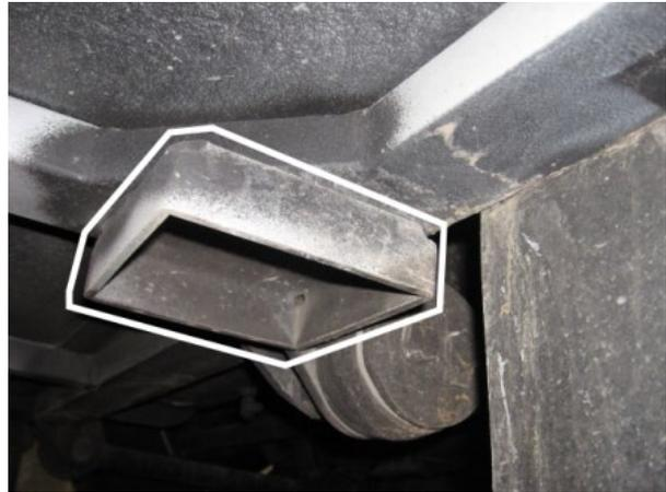
**FIGURE 16: SUPPORT DE LEVAGE AU CHÂSSIS
