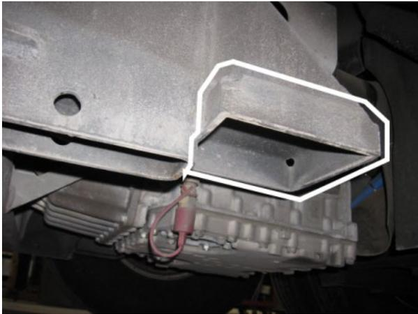
**FIGURE 15: SUPPORT DE LEVAGE AU CHÂSSIS
