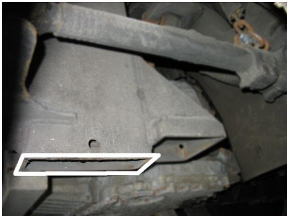
FIGURE 3: POINTS DE LEVAGE DU CHÂSSIS
