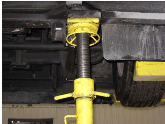
**FIGURE 18: CHANDELLE AU SUPPORT DE LEVAGE -
