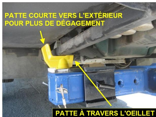
**FIGURE 62: EMPLACEMENT RECOMMANDÉ POUR LE
