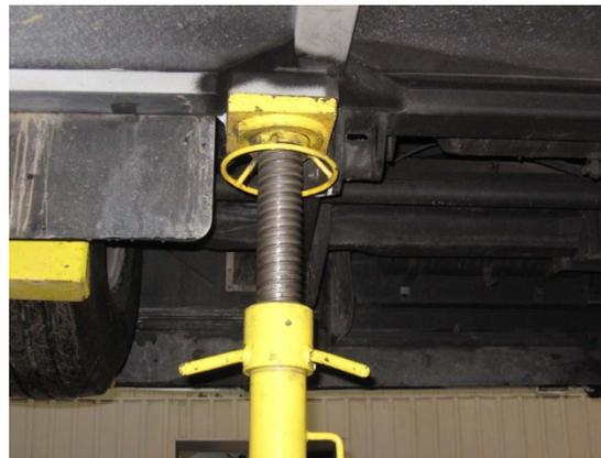
FIGURE 4: CHANDELLE AU POINT DE LEVAGE DU
