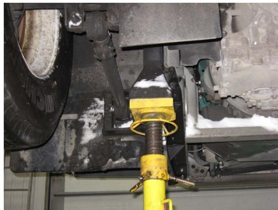
**FIGURE 20: CHANDELLE AU SUPPORT DE LEVAGE -
