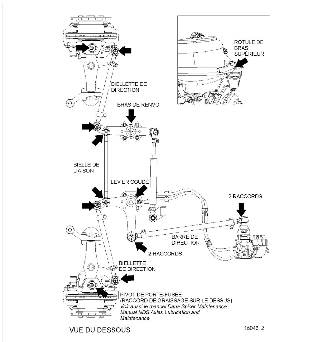
FIGURE 1 : POINTS DE LUBRIFICATIONS - SUSPENSION INDÉPENDANTE (TYPIQUE)
